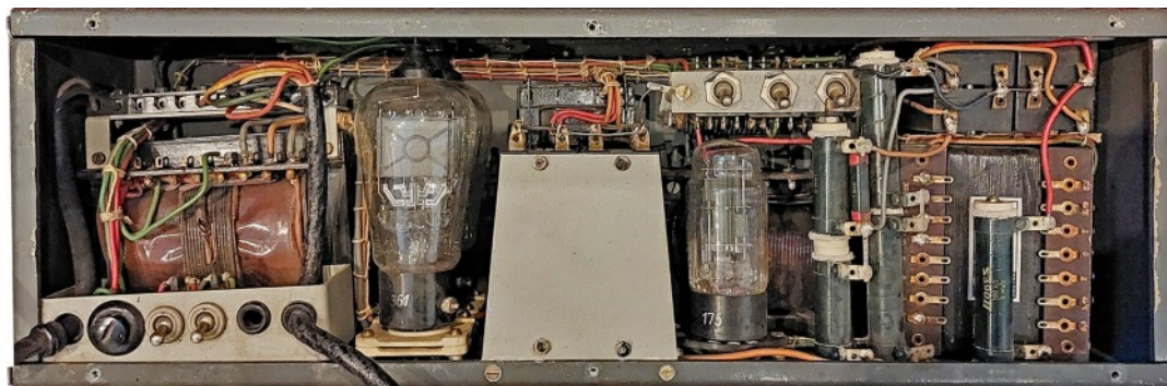
Front view of GI 89 power supply unit with front cover detached.
